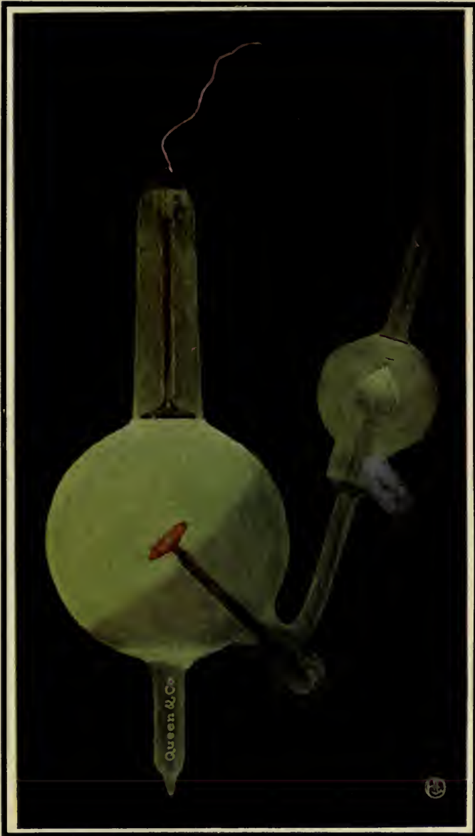
SELF-REGULATING X-RAY TUBE. OPERATING PROPERLY.
