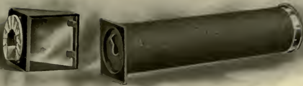
FIG. 217.—The improved benoist radiochromometer.
