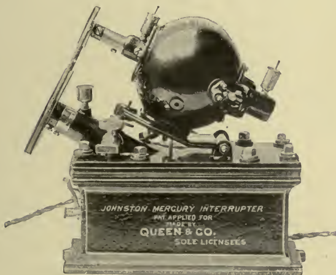
FIG. 73.—Johnston's mercury interrupter.
