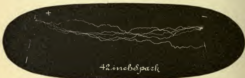
FIG. 103.—The polarity as determined by the appearance of the spark.
