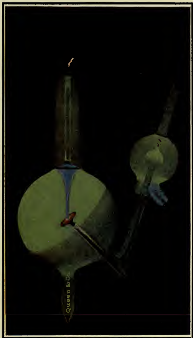
SELF-REGULATING X-RAY TUBE. LOW VACUUM. (Fig. 96.)
