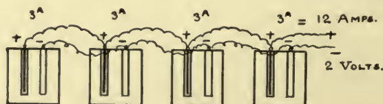
FIG. 3.—Connection of the cells in "parallel."
