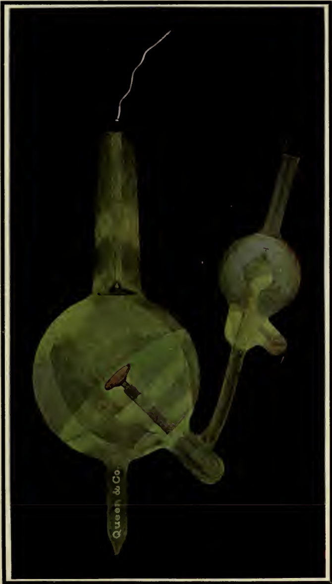
SELF-REGULATING X-RAY TUBE. CURRENT RUNNING IN WRONG DIRECTION.
