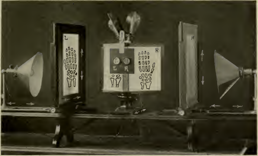
FIG. 114.—Wheatstone's reflecting stereoscope, as modified by Weigel.
