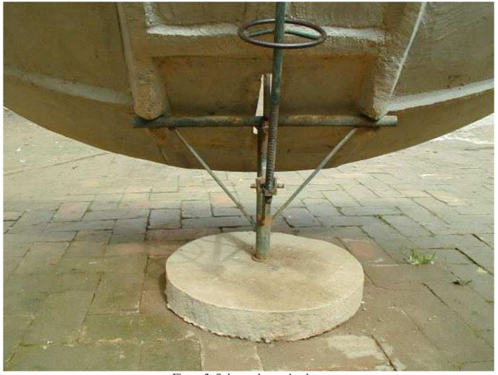
Figure 2: Solar cooker underplate.
