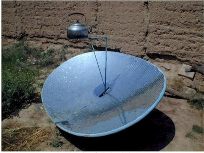
Figure 1: A solar cooker heating a kettle of water.
